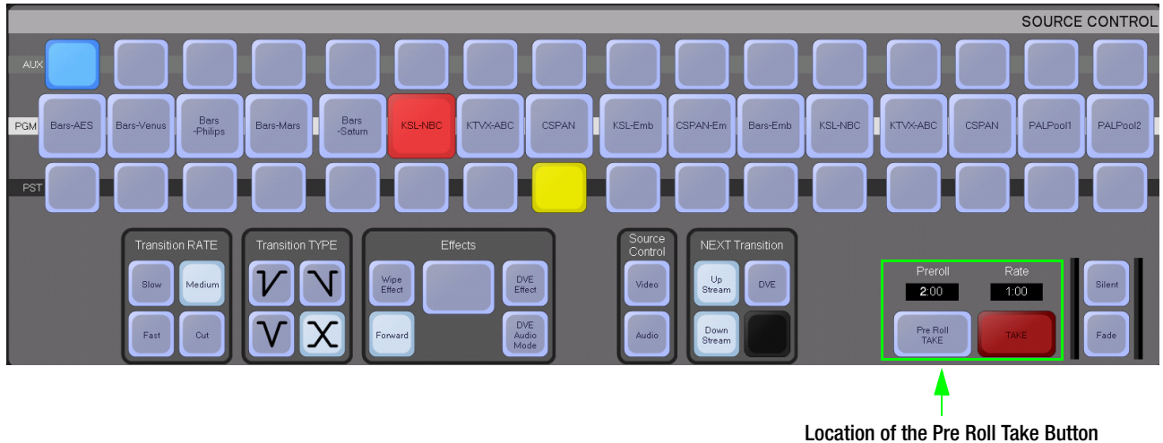
Figure 13. Location of the Pre Roll Take Button in the Source Control Section
